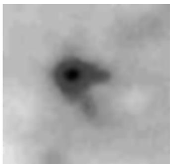
Fig 4: The electron beam transverse profile produced when a short laser pulse breaks up in plasma corresponding to the figure above.
