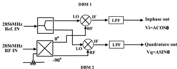
Figure 3: Block diagram of the fast phase detector (IQ detector).
