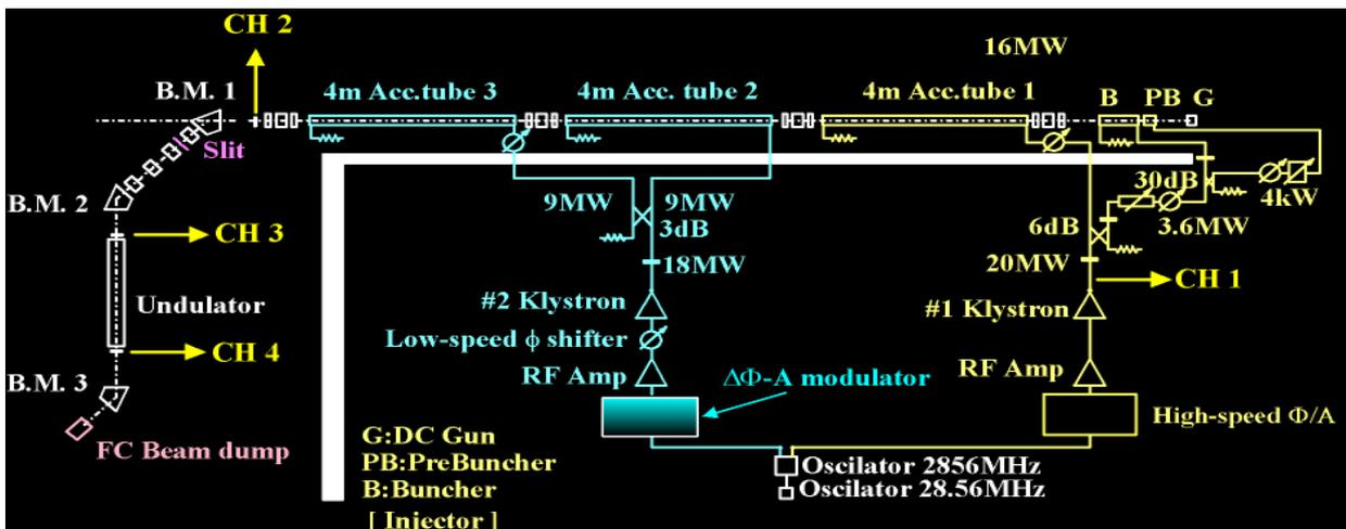
Figure 4: Experimental setup for  $\Delta\phi$ -A initial beam loading compensation system.
