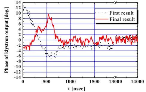
Figure 7: Result of klystron output (phase).
