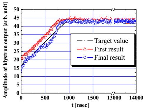
Figure 5: Result of klystron output (amplitude).
