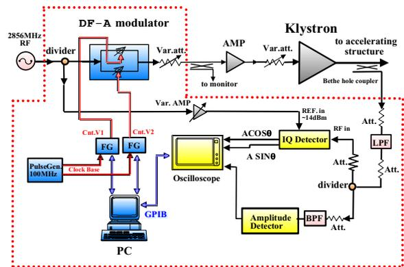
Figure 1: Block diagram of the  $\Delta\phi$ -A modulation system for initial beam loading compensation.
