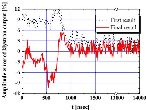
Figure 6: Result of klystron output error (amplitude).
