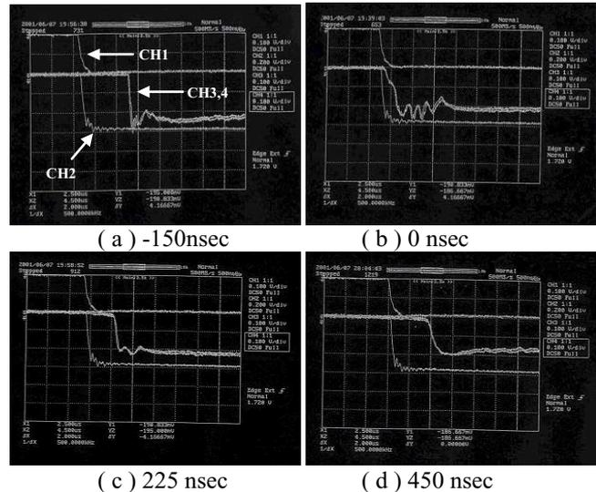
Figure 8: Measured beam pulse waveform with different injection timings. CH1 shows the amplitude of #1 klystron output. CH2 shows the beam waveform at the end of straight section. CH3 and CH4 show the beam waveform before and after the undulator respectively. Electron beam is injected after one filling time (b). (a), (c) and (d) are the case of beam injected timing being delayed to the first filling time for -150nsec, 225nsec and 450nsec respectively.
