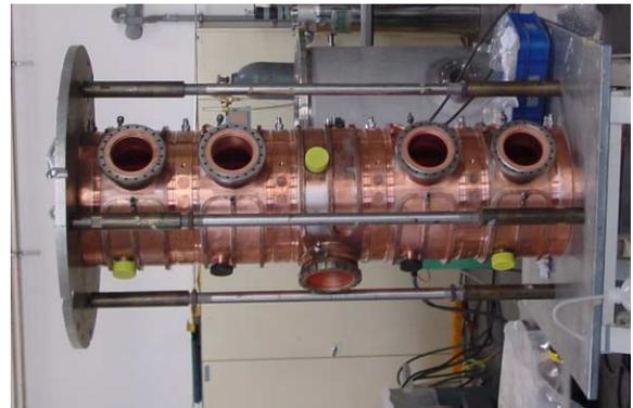
Figure 3: Five-cell cavity (by courtesy of Accel GmbH).
