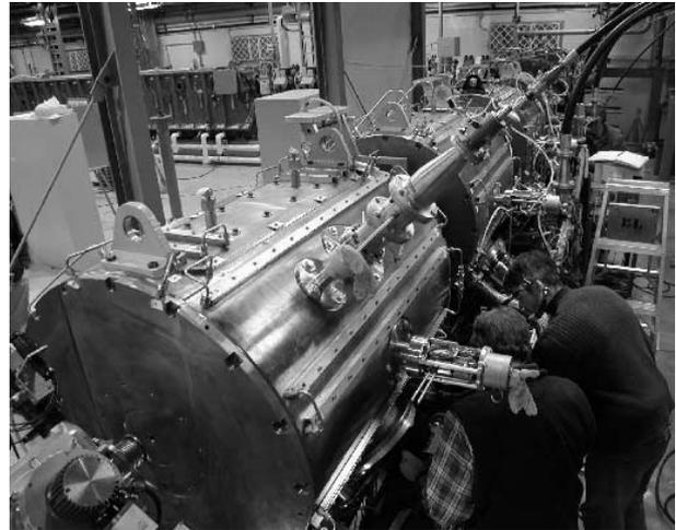
Figure 2: The ISAC 106 MHz DTL.
