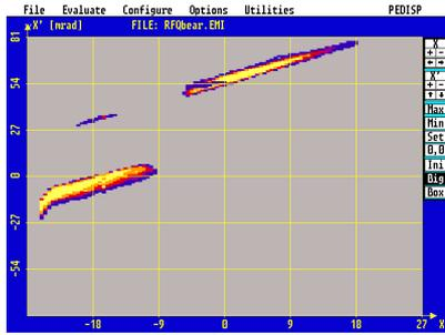
Fig. 8: Emittance measurement with the deflector switched off.
