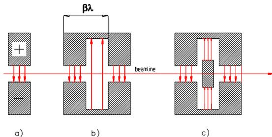
Fig. 5: Schemes of funnel deflectors. The arrows show the electric field during one period. a) a one cell one gap deflector, b) a three cell multigap deflector, c) multigap deflector with one central drift tube.
