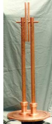
Fig. 6: Picture of the one gap funnel deflector. The deflector discs are mounted at water-cooled stems. The height is about 2 m.
