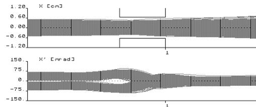
Fig. 7: Simulation of the beam bending in the one gap funnel deflector. The rectangles are the deflector plates (top picture), the lower picture shows the beam bending from 38 mrad down to zero.
