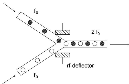
Fig. 1: Principle of funneling.
