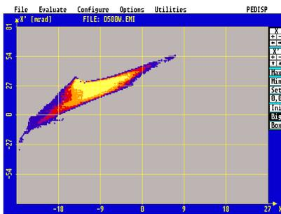
Fig. 9: Emittance measurement with the one gap deflector switched on. The two emittances are merged into a common beam.
