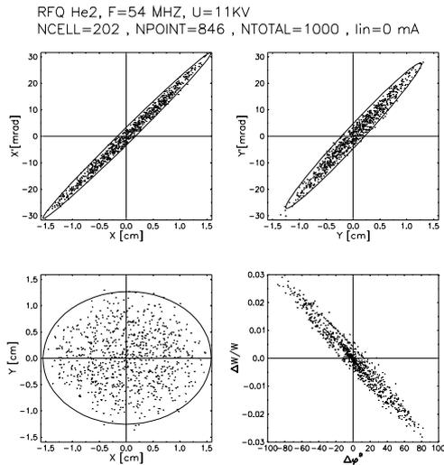
Fig. 3: Beam data of the funneling deflector with actual RFQ.
