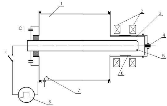
Figure 5: Scheme of the experimental setup. 1. capacitance-loaded quarter-wave resonator; 2. solenoid; 3. tungsten-wire thermionic cathode; 4. feed input; 5. central resonator electrode – diode anode; 6. working area of secondary emission cathode; 7. excitation loop/diagnostics; 8. pulsed high-voltage generator; C1 blocking condenser
