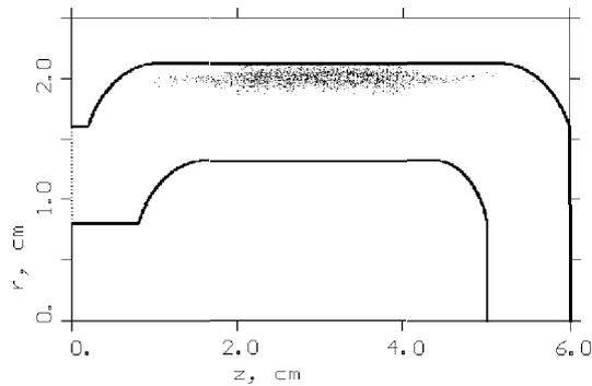
Figure 3: Gun geometry.
