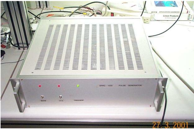
Figure 8: Picture of SRRC-1000 Thyatron trigger system.
