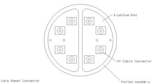
Figure 9. View of potted, split rod secondary assembly.
