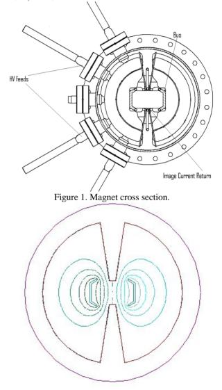
Figure 2. Cross section and flux lines in magnet.
