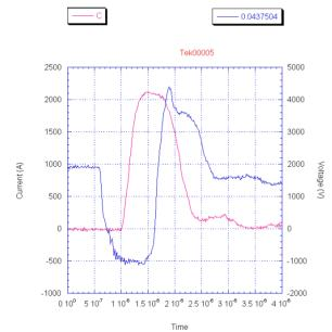
Figure 8. Current pulse and core voltage with four pipe secondary design.
