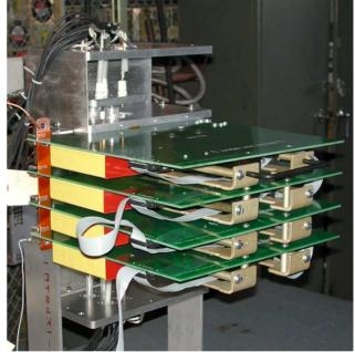
Figure 6. Photo of four stack proto type modulator.
