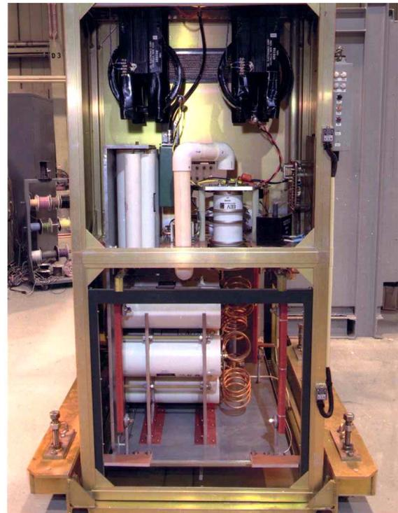
Figure 1. The RHIC Beam Abort Kicker High Voltage Modulator.
