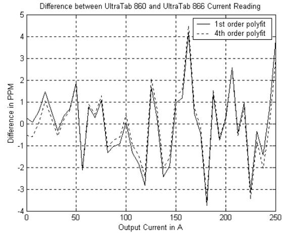
Figure 3. Current difference between standard device and device to be calibrated.
