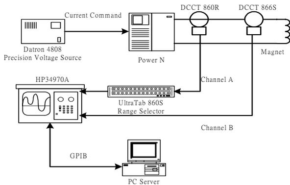
Figure 2. calibration Set-up of Measurement device.
