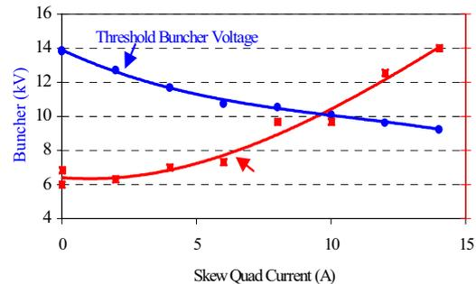
Figure 7. Instability threshold voltage and relative beam losses as a function of skew quad current for fixed beam intensity (stored charge of 5 µC/pulse).
