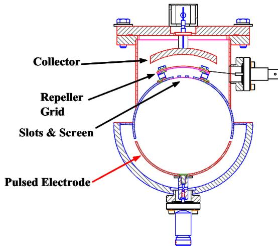
Figure 5. Cross-section of the electron sweeping detector.
