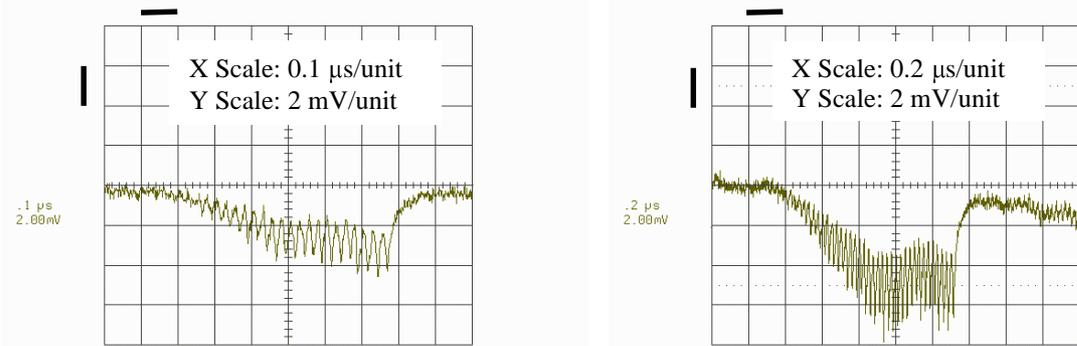
a) Pick-up signal for a bunch intensity of  $6.9 \times 10^{10}$  p/b      b) Pick-up signal for a bunch intensity of  $8.3 \times 10^{10}$  p/b
