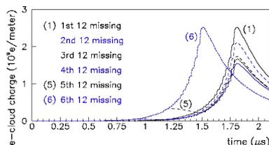
Figure 5: Simulated evolution of electron cloud line density in unit of  $m^{-1}$ , as function of time during the passage of the bunch train through a field-free region in TT2. The six possible cases of 12 missing bunches are represented. The total bunch length is 4 ns, and elastic electron scattering is taken into account.
