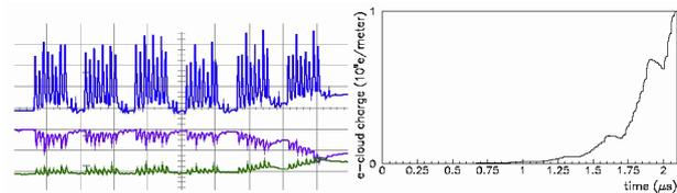
Figure 6: (left) Measured baseline drift in a TT2 electrostatic pick-up with 6 gaps of 120 ns. From top to bottom,  $\Sigma$ ,  $\Delta x$ , and  $\Delta y$ . Time scale: 200 ns/div. (right) Corresponding simulated electron line density.
