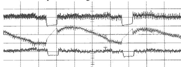
Figure 1: Measured baseline drift in a PS electrostatic pick-up during bunch compression prior to extraction. From top to bottom,  $\Sigma$ ,  $\Delta y$ , and  $\Delta x$ . Time scale: 500 ns/div. The 30 MHz bandwidth of the pick-up does not allow to discriminate the 4 ns bunches. The bunch train lasts  $1.8 \mu\text{s}$  and the gap is 320 ns.
