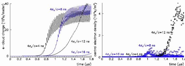
Figure 3: Simulated evolution of electron cloud line (left) and central (right) densities in units of  $m^{-1}$  and  $m^{-3}$  respectively, as function of time during the passage of the 72 proton bunches through a PS dipole chamber. Four bunch lengths (4, 8, 12, and 16 ns) are considered, taking into account elastic electron scattering.
