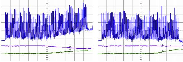
Figure 2: Measured baseline drift in a TT2 electrostatic pick-up: solenoid OFF (left) and ON, with about 50-100 Gauss, (right). From top to bottom,  $\Sigma$ ,  $\Delta x$ , and  $\Delta y$ . Time scale: 200 ns/div. This pick-up has a larger bandwidth than the one of Fig. 1, which allows to discriminate the short bunches. The bunch structure is not observable on  $\Delta x$  and  $\Delta y$  signals, as the beam is centred in the pick-up.
