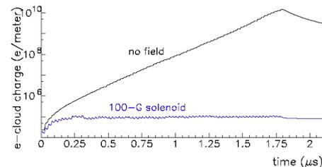
Figure 7: Simulated electron cloud line density in a TT2 field-free region, without and with a solenoidal field of 100 Gauss.
