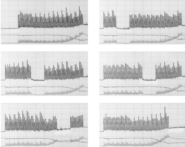
Figure 4: Measured baseline drift in a TT2 electrostatic pick-up, with the six possible cases of 12 missing bunches (i.e. one PS-Booster ring). From top to bottom,  $\Sigma$ ,  $\Delta x$ , and  $\Delta y$ . Time scale: 200 ns/div.
