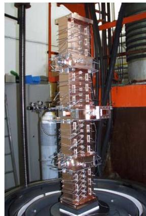
Figure 3: LIBO prototype in the oven for the penultimate brazing
