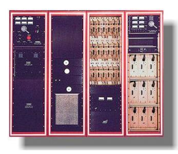
55-Kilowatt Single Tube Tetrode RF Amplifier designed and built for Duke University FEL
