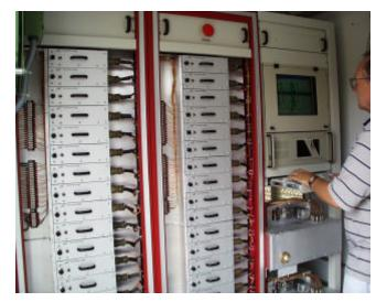
20 KW, 27 mHz, Solid-State Trailer Mounted (Mobile) Generator designed and built for KAI Technologies
