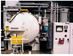
A view of one of Fremont's high temperature vacuum furnaces shown with the cryogenic vacuum pump and Honewell controls and recorders.
