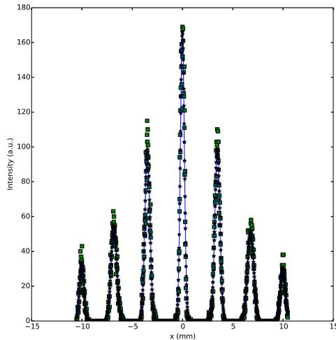
Figure 4: The horizontal projection of the beam stripes on the profile monitor for beam energy of 2.6 MeV, and the multiple Gaussian peak fitting of the projection.
