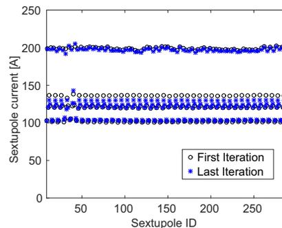
Figure 6: Topup mode, sextupole magnets strength for the first and last iteration, a total of 280 sextupoles in 40 sectors (21 families in total). Starting point is optimized sextupoles from MOGA simulation [7] on the medium chromaticity lattice ( $\xi = 6$ ).
