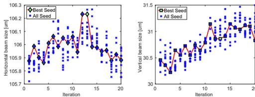
Figure 3: Horizontal and vertical beam size (at sector 35 pinhole location) for each iteration. A total of 20 iterations, and 10 seeds for each iteration. Starting point is optimized sextupoles from MOGA simulation [7, 15] on the high chromaticity lattice ( $\xi = 11$ ).
