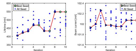
Figure 5: Topup mode, lifetime (left) and beam current (right) at each iteration. A total of 10 iterations, and 10 seeds for each iteration. Starting point is optimized sextupoles from MOGA simulation [7, 15] on the medium chromaticity lattice ( $\xi = 6$ ).
