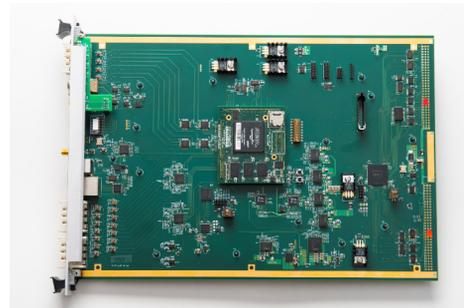
Figure 1: An example of a SoC MFC Board.
