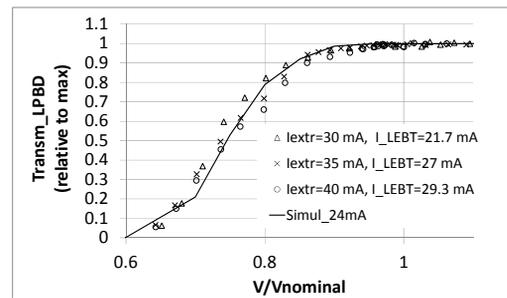
Figure 6: Relative transmission to LPBD vs RFQ voltage.
