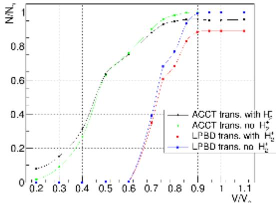
Figure 3: simulated transmission trough RFQ with/without contaminants for 8 mA input current [4].
