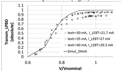
Figure 5: Absolute LPBD transmission vs RFQ voltage.
