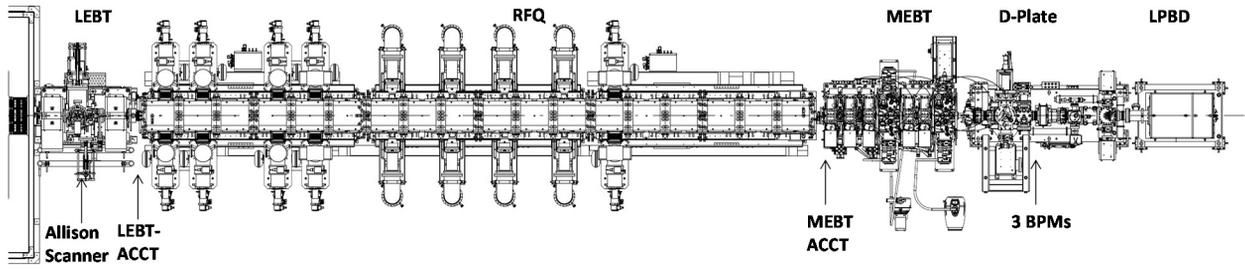
Figure 2: LIPAc configuration showing main systems and diagnostics mentioned in this paper.
