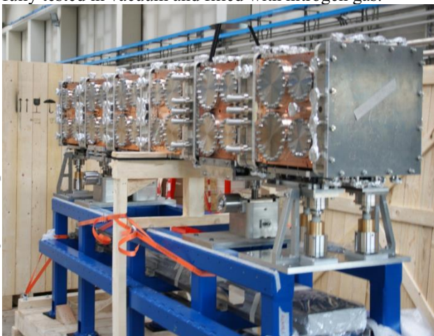
Figure 2: Assembly of the SM in the wooden box before shipment.
