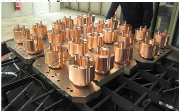
Figure 5: Semi-finished copper tuners ready for brazing at LNL furnace.
