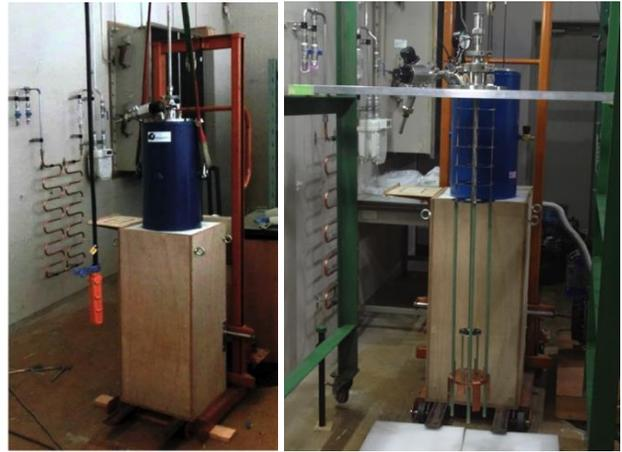
Figure 6: The cryostat and the heat exchanger for He gas return system on the wall (left).
