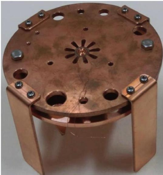
Figure 5: Test coil put in a Cu plate of the cryogenic stage.
