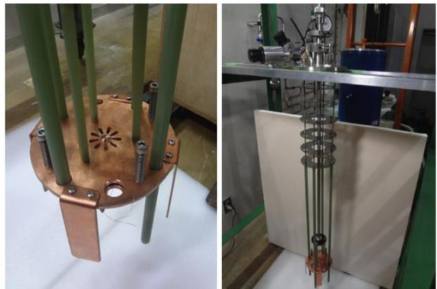
Figure 7: The cryogenic stage hung by FRP rods (left) and its overview (right) in front of the cryostat.
