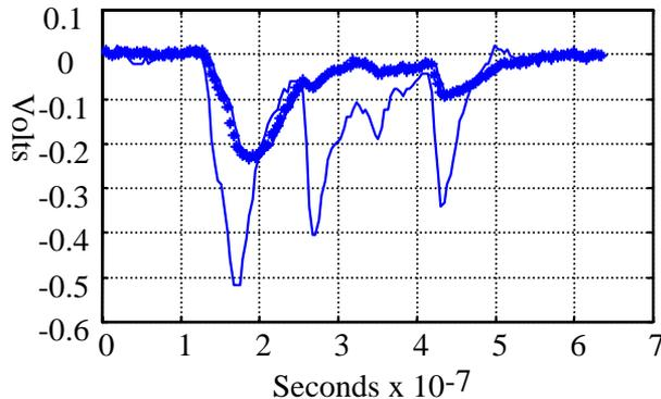
Figure 3: Loss monitor signals, (recorded during 1.2 GeV SLC beam operation), showing the difference between the Ar/CO<sub>2</sub> (95/5%) gas mixture (\*) and the Ar/CF<sub>4</sub> (90/10%) gas mixture (-)[6]. The figure shows CCLM signals from a beam loss of about  $4 \times 10^9$  particles distributed over three locations (0.8J total). The CCLM was mounted 0.3 m from the beamline.
