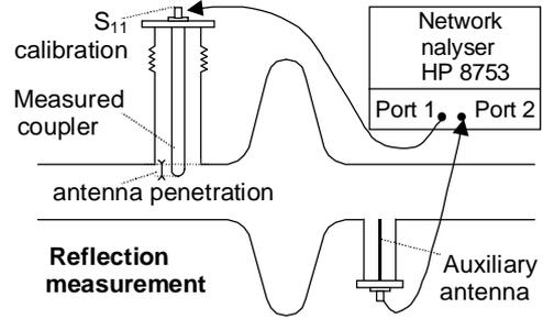
Fig. 3. Qext measurement in the 1-cell copper mock-up.
