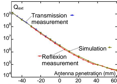
Fig. 4. Computed and measured  $Q_{ext}$  in the mock-up.
