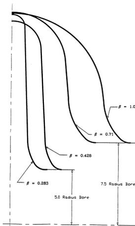
Fig. 5. Shapes of half cells for different  $\beta$ .
