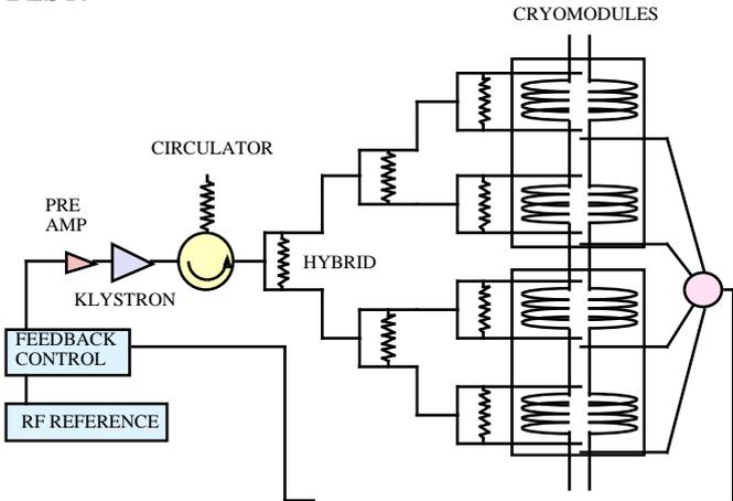
Fig. 4. RF system architecture.
