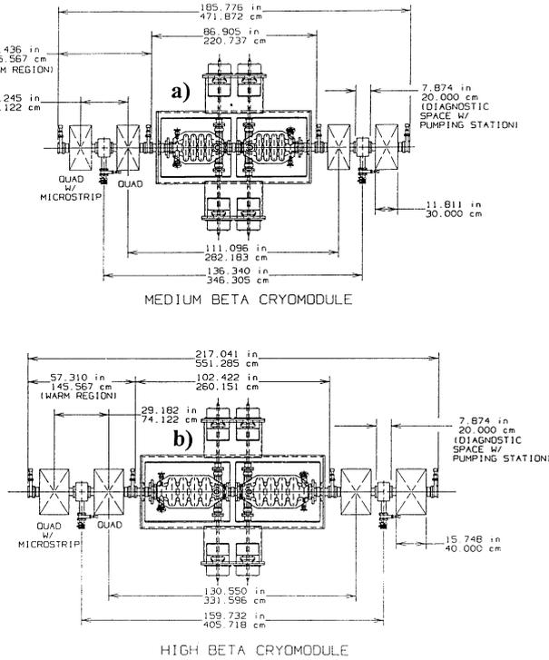
Fig. 2 Layout of a) medium- section, b) high- section.
