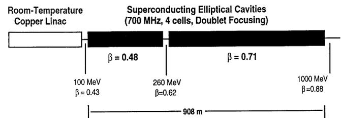
Fig. 1 Schematic layout of the APT SCRF linac
