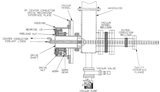
Fig. 3. Schematic of power coupler.
