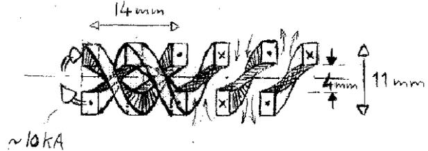
Figure 1 Diagram of an iron free helical undulator. (Picture courtesy of S.L. Wipf.)
