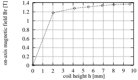
Figure 4. Radial magnetic field amplitude  $B_r$  as function of the coil height  $h$  with constant inner radius  $r_i$  of 2mm.
