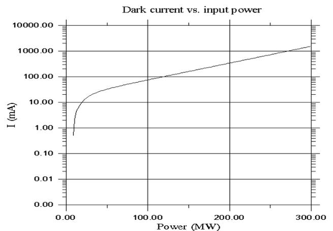
Fig. 1 Dark current vs input power
