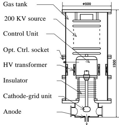
Fig. 2. The electron gun layout.
