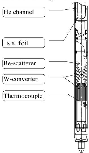
Fig. 3. Basic target-converter elements.
