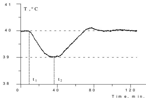
Fig. 4. The temperature of the accelerating section. At the moment  $t_1$  the thermal mode was changed from 40°C to 39°C, and at the moment  $t_2$ , it was returned to 40°C
