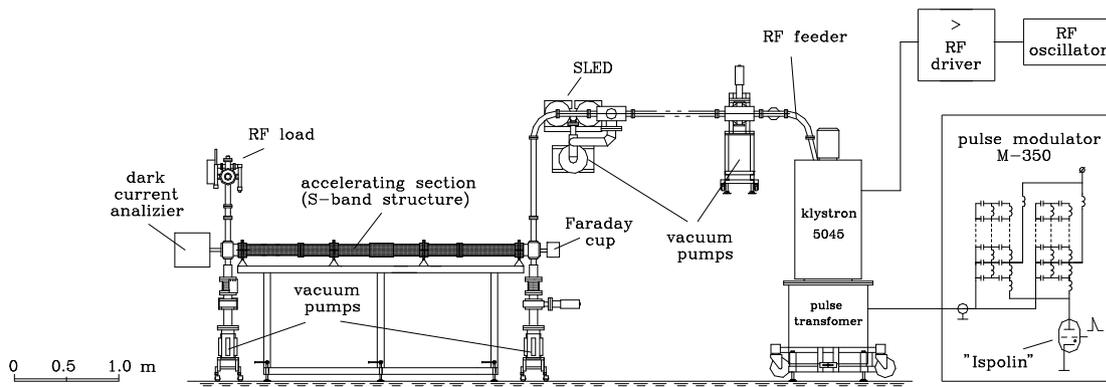
Fig. 1. The IREN Full-Scale Test Facility layout
