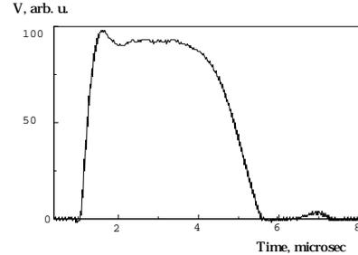
Fig. 2 The shape of the M-350 PFN voltage pulse. (preliminary result).
