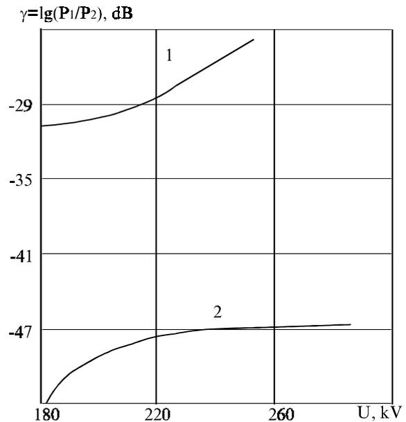
Fig.4. The relative level of the second harmonic power as a function of the anode voltage in the supplementary output cavity (curve1) and at the exit of a standard klystron (curve2).
