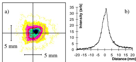
Fig. 7. a) Image of the beam focal spot on a phosphor screen positioned at the RFQ input plane (recorded using a gated CCD camera)
