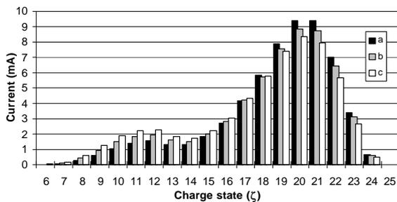
Fig. 3. Charge-state distribution of the unaccelerated plasma. Measured data processed under the assumption that a) the secondary electron emission coefficient ( $g$ ) of CuBe is independent of charge-state and kinetic energy, b)  $g$  scales with ion kinetic energy, c)  $g$  proportional to charge-state.
