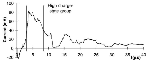
Fig. 4. Beam current measured with a 30mm aperture Faraday cup positioned 24 mm after extraction. High charge-state Ta beam is indicated from 3-8  $\mu$ s after the laser pulse.
