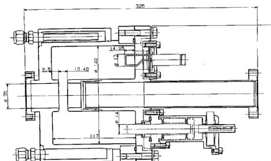
Fig. 3. Structure of SHB2 cavity.
