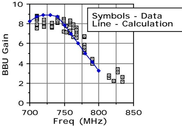
Fig 2 Measured & calculated BBU gain thru ITS cell-block
