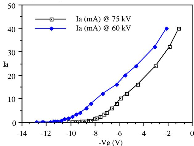
Fig. 1 Gun emission curves at 60 and 75 kV.
