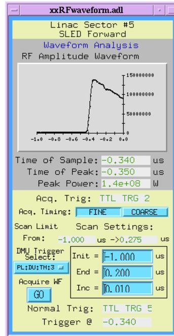
Fig. 2. A typical SLED waveform timescan.
