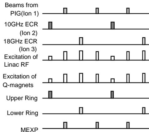
Fig. 3. Beam-pulse relation in the TSA system.
