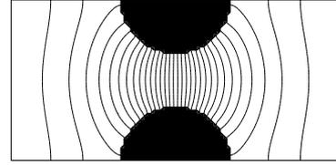
Figure 5: Fundamental mode.  $\beta = 61.83 \text{ m}^{-1}$ .
