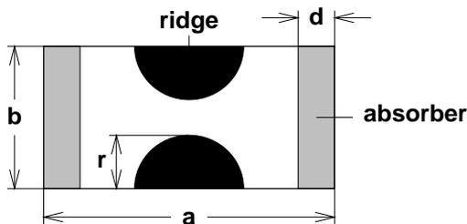
Figure 4: Cross section of a ridge waveguide with circular ridges and absorbers at the side walls.
