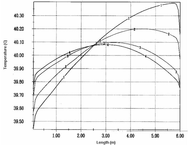
Fig. 4 : Surface temperature with optimised inlet water temperature in order to cancel the sum of the single cell phase error towards the end of the structure
