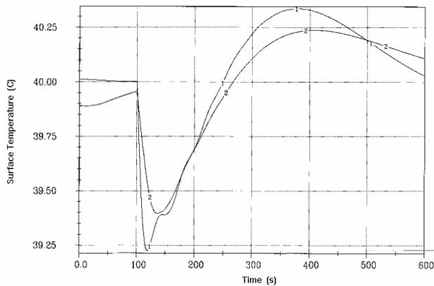
Fig. 6 : Temperature of the surface by changing the repetition frequency from 50 Hz to 10 Hz
