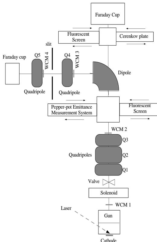
Figure 1: CANDELA beamline showing diagnostics devices
