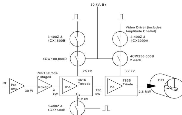
Fig. 1. Original 201 MHz Amplifier System.
