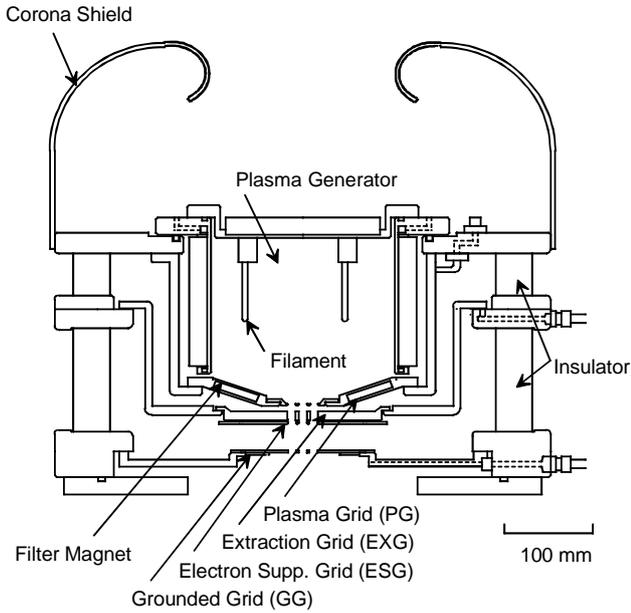
Fig. 2. Cross sectional view of the multi-aperture volume type negative ion source
