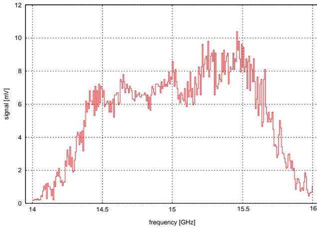
Fig. 4: Dipole mode spectrum observed at a horizontal HOM-output coupler, while the beam was steered to a vertical offset of 1.3 mm. Spectra were taken over a 30sec sweep time, with 2GHz span, and 1 MHz resolution bandwidth, at a beam rate of 50Hz.
