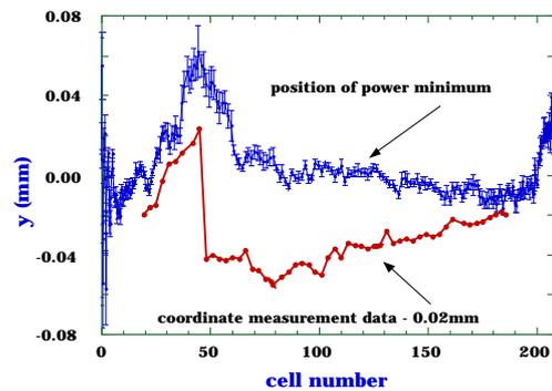
Fig. 6: Comparison of a structure-straightness measurement (lower curve) with the microwave-based determination of the electrical center. The 60  $\mu\text{m}$  kink in the structure is reproduced in the minimum power-position measurement, though smeared out somewhat due to the fact that the modes extend over a fair number of cells.
