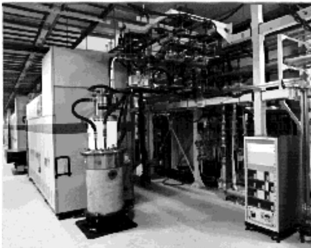
Fig.3 RF-source upgrade of the existing linac for KEKB: the modulator powers were doubled; the PFN cabinets became tall-boy in order to make a capacitance doubling; and the klystron outputs were upgraded from 30 MW to 50 MW while maintaining the height.
