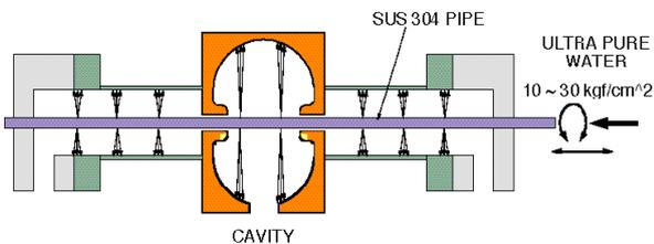
Fig. 10. Cavity rinsing procedure by high pressure ultra pure water.
