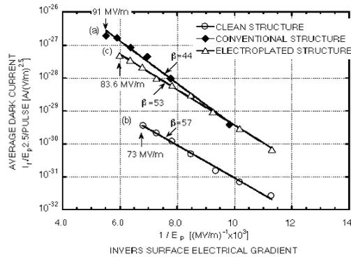
Fig. 2. Modified Fowler-Nordheim plots for three 60 cm-long traveling-wave structures.
