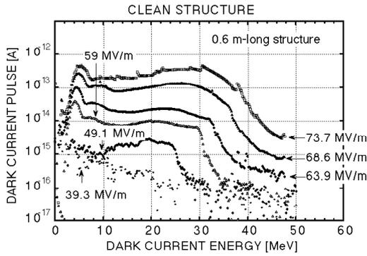
Fig. 3. Dark current energy spectrum of the clean structure.
