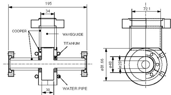
Fig. 5. Three TM<sub>010</sub> cavity dimensions. Only the Ti bounded cavity has Ti blocks around the beam holes.
