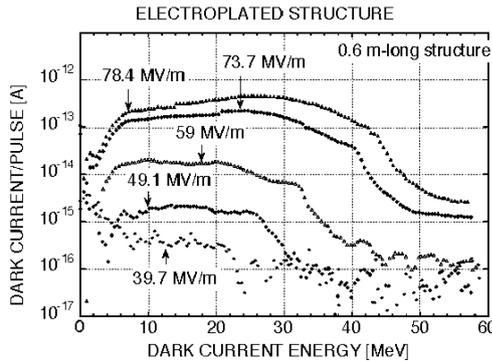
Fig. 4. Dark current energy spectrum of the electroplated structure.
