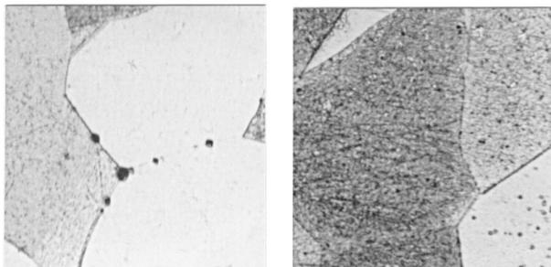
Fig. 6. Optical micrographs showing forged OFHC copper (left) and HIP-OFHC copper (right). [HIP parameters: temperature 850 °C and isostatic pressure 1200 kgf/cm<sup>2</sup>].
