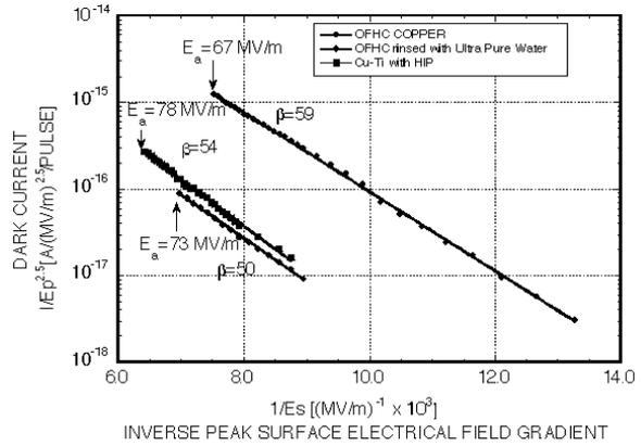
Fig. 7. Modified Fowler-Nordheim plots for the three differently processed cavities.
