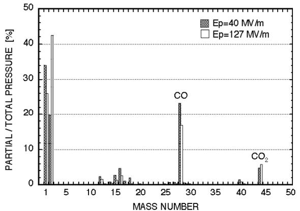
Fig. 8. Residual gas mass spectrum of the conventional cavity during rf power tuning.
