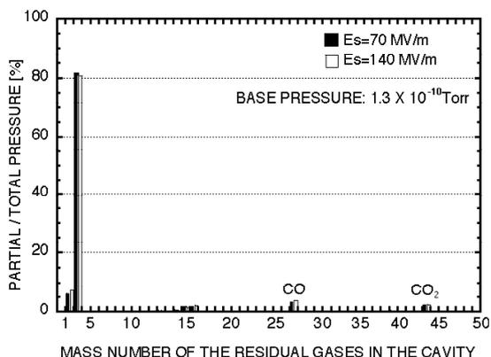
Fig. 9. Residual gas mass spectrum of the clean cavity during rf power tuning.
