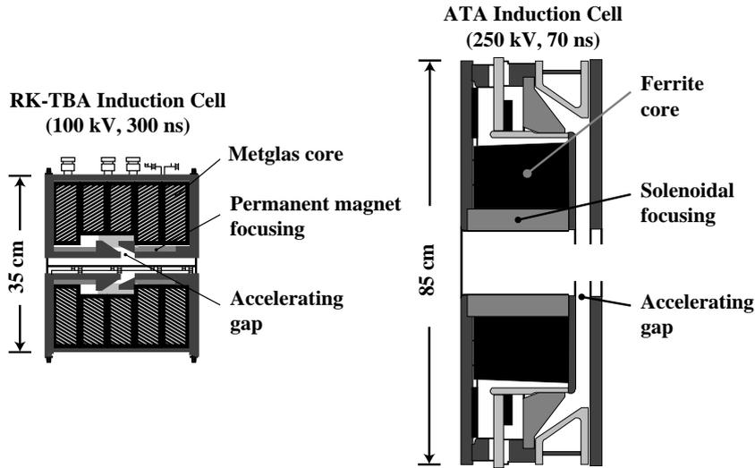
Figure 1. The RTA cell (100 kV, 300ns) is much more compact than the ATA cell (250 kV, 70 ns).
