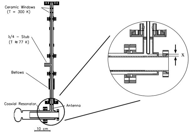
Figure 2: Cut of the tuneable sc input coupler.
