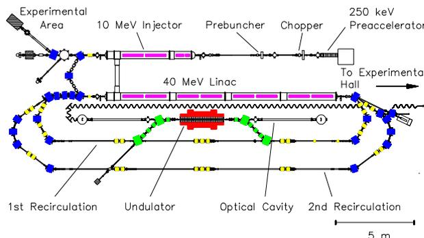
Figure 1: Layout of the S-DALINAC accelerator hall.
