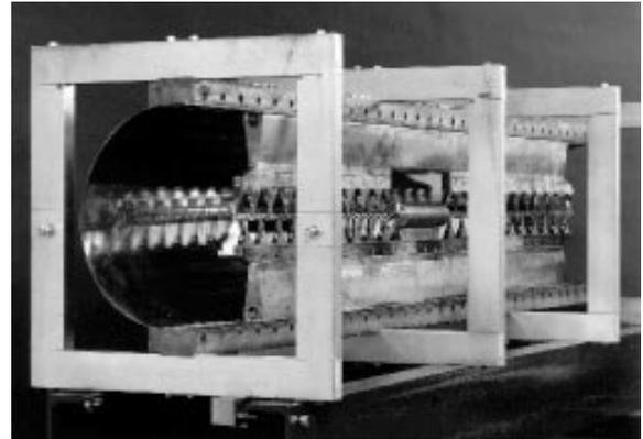
Figure 5: The 1:5.88 model for cavity IH2 (Photo: A. Zschau, GSI).
