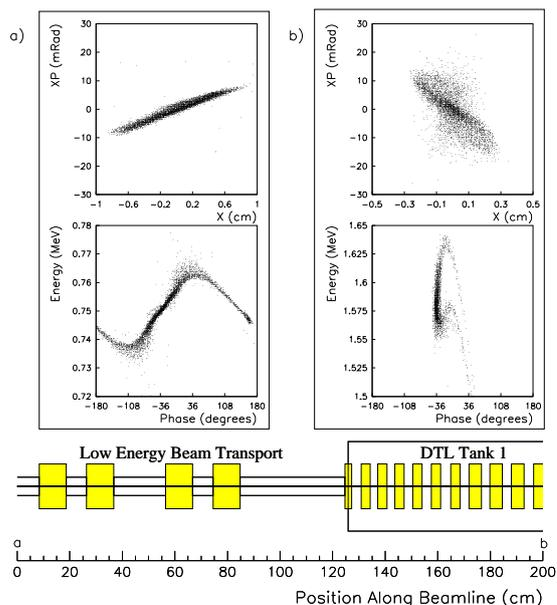
**Fig. 1:** (a) The horizontal and longitudinal phase-space distributions at the last emittance measuring station and (b) at the exit of the tenth drift tube for the standard quad and buncher settings. The bottom schematic diagram shows the end of the LEBT and the entrance to the DTL (shaded blocks are quadrupole magnets).
