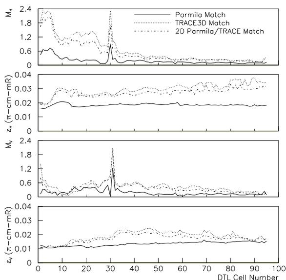
**Fig. 3:** Horizontal and vertical mismatch ( $M$ ) and normalized emittance ( $\epsilon$ ) versus drift tube number in the first two tanks of the DTL.
