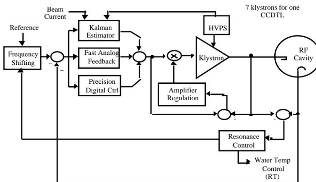
Fig 2. Block diagram of the LLRF control system.
