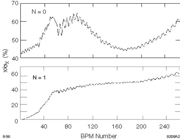
Fig. 2: The normalized jitter in the linac is not constant for high current, but can grow or damp depending on the BNS damping setup. A typical SLC behavior is shown at the top ( $N = 0$ ), while a higher order jitter ( $N = 1$ , bottom) is invisible with a normal BPM at the beginning, but then grows to the same amplitude.
